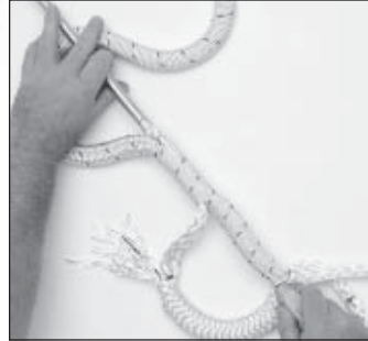
Pushing fid and core through cover
