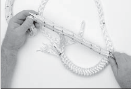
Inserting fid through cover
