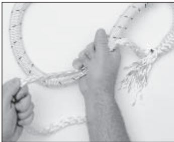
Pulling core end to tighten cross-over
