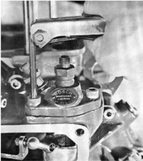
11. Remove the governor by loosening the hexagonal set screw (1), the governor and the gear wheel can then be withdrawn.
