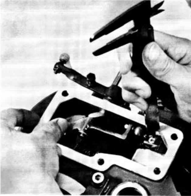
**75.** If the engine smokes abnormally, the centre screw on the cover can be loosened and the adjusting screw can be adjusted until the engine runs smoke free. See the technical data for the correct injection amount.
