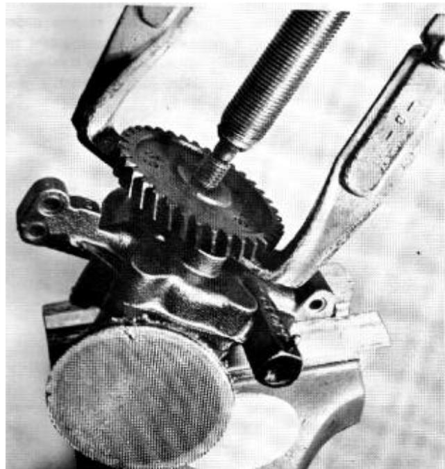
21. Remove the steel wire which holds the filter. Remove and clean the wire gauze thoroughly. Afterwards remove the six screws which hold the cover in position. Discard the gasket.
