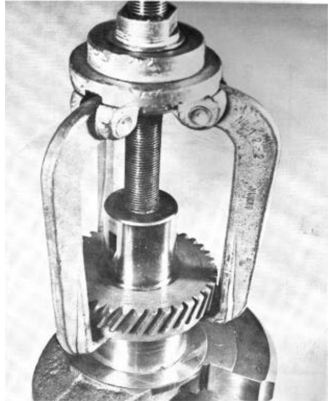
**36.** Place the key in the crankshaft's key slot. Heat the gearwheel to approximately 100°C (212°F) (no more) and press it onto the crankshaft. Note! The marking on the gearwheel shall face outwards. Refit the circlip on the crankshaft.
