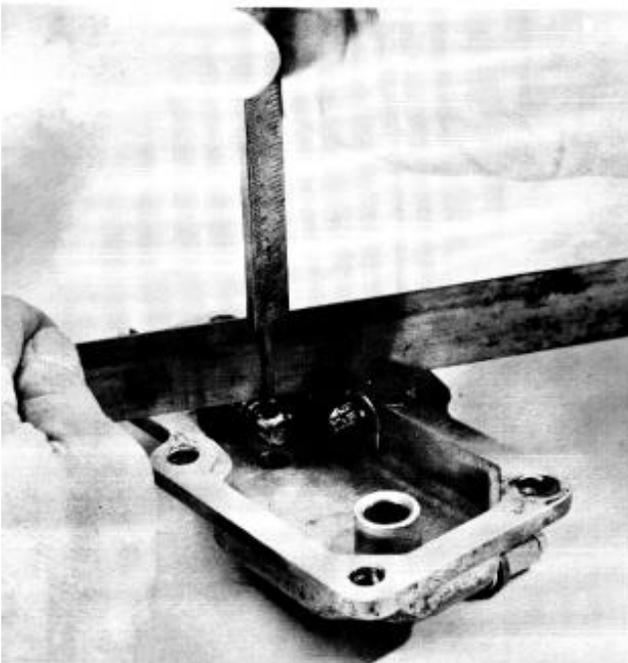
**76.** Fit a new gasket and fit the flywheel cover. Be careful so that the sealing ring is not damaged. Trim the excessive gasket.
