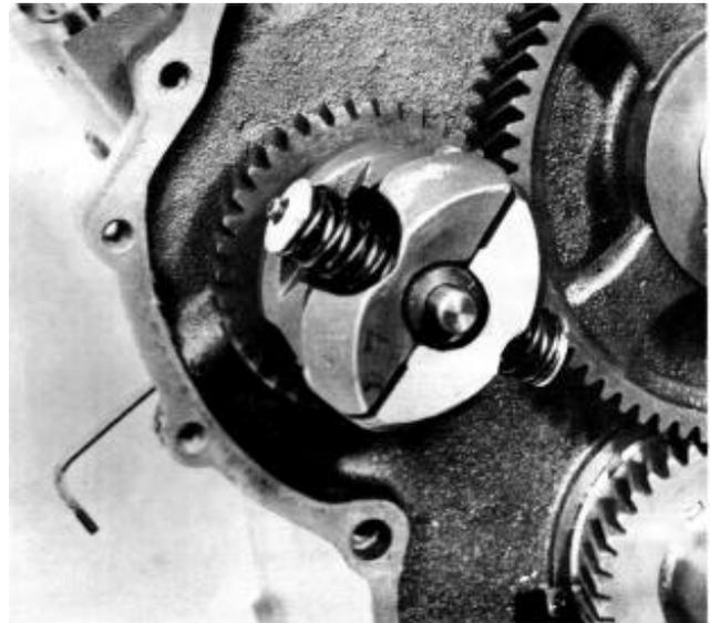
69. Fit the gearwheel on the camshaft's opposite end.
