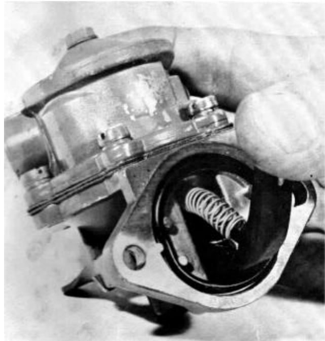
29. Remove the cover's centre screw, remove the filter 1 and clean it.
