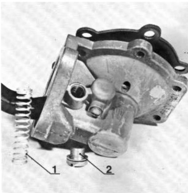
32. Remove screw 1 and withdraw the manual pump arm 2 and replace spring 3 if it is broken. Note! Be careful of the rubber seal which is pressed into the housing.
