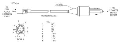
**Power Data Adapter Cable** - allows access to serial port and NMEA interface for GPS operations and the RS-232 data download cable that ships with the unit.
