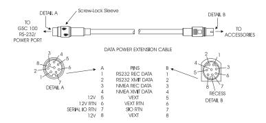
To connect to external power, connect the screw-lock sleeve, shown above, to the RS-232/Power port on the side of the GSC 100. Take the AC power adapter cable, shown on the following page, and snap it onto the available end of the data power extension cable. Make sure that the connections are snug so as not to disconnect during use. The AC power adapter cable is now ready to plug into external power.
