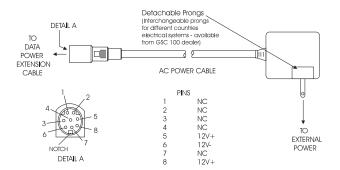
To connect the RS-232 software update cable, connect the screw-lock sleeve on the data power extension cable, shown on the previous page, to the RS-232/Power port on the side of the GSC 100. Take the RS-232 software update cable, shown below, and snap it onto the available end of the data power extension cable. Make sure that the connections are snug so as not to disconnect during use. The RS-232 software update cable is now ready to connect to the 9-pin serial port on your PC.
