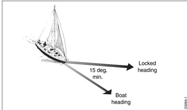
The value must be within the range 15 to 40°, and can be adjusted in 1° steps.
