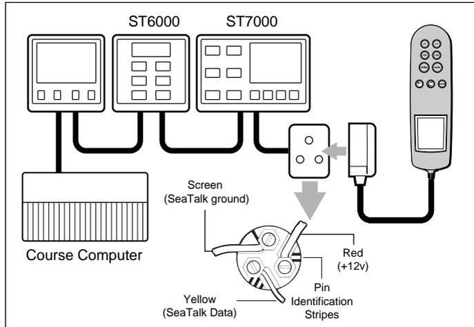
Note: The hand held socket can be installed anywhere on the SeaTalk bus.
