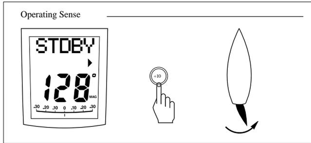
3. If the helm produces a turn to port, reverse the motor connections at the course computer.
