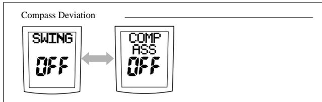
4. Press the **+1** or **-1** key to change the setting from OFF to YES. The Turn Boat page is then displayed after 1 second.
