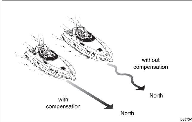
The patented AutoAdapt feature allows the autopilot to compensate for heading errors at higher latitudes, which are caused by the increasing dip of the earth’s magnetic field. The increased dip has the effect of amplifying rudder response on northerly headings in the northern hemisphere, and on southerly headings in the southern hemisphere.
