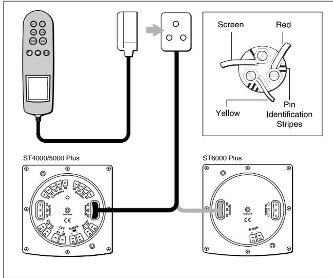
The ST600R can also be connected to any available SeaTalk instrument as well as the autopilot.
