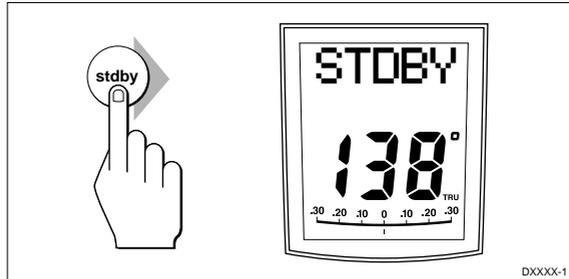
This shows that the control head is active. If the unit does not beep, check the fuse/circuit breaker.
