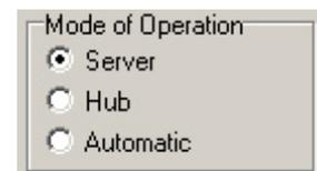
**Server mode:** In this mode, the combination of computer and multiplexer acts as an NMEA server. Incoming NMEA data from NMEA In1 to In4 is sent to the computer on the USB port. Only NMEA data from the computer is available on NMEA Out2.
